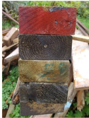
Arsenic and Old Wood ^ > Pressure treated wood sold before 2004 may contain CCA, a hazardous chemical compound containing arsenic.
